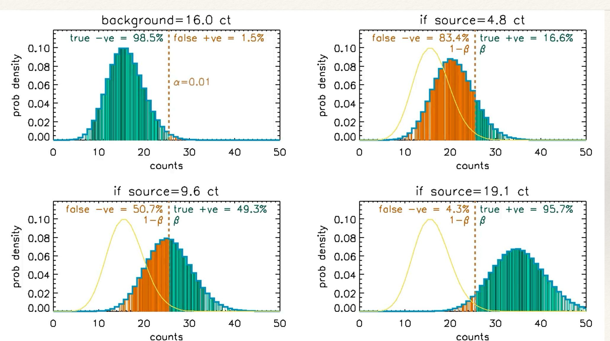
When no signal is detectable, it is useful to know what is the maximum brightness that a source could have at which point it would be detected.
