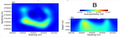
Identifying and delineating geologic units based on multiple physical property models obtained from geophysical inversions.
