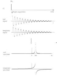
Fig. 2.7 Free Induction Decay (F1D) following a single 90° r.f. pulse. The real and imaginary parts of the signal correspond to the in-phase and quadrature receiver outputs. The signal is depicted with receiver phase  $\phi = 0$  and, on complex Fourier transformation, gives real absorption and imaginary dispersion spectra at the offset frequency,  $\Delta \omega = \omega_0 - \omega$ .
