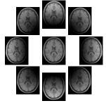
8-coil system (noiseless situation): Images from receiver coils and combined image
