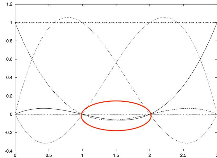
region of interpolation ( $\mathbb{P}_3$  finite elements and cubic Lagrange)
