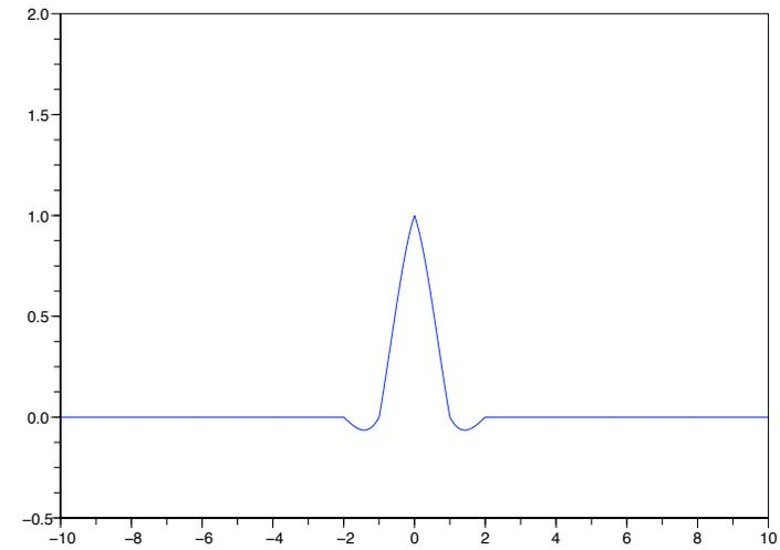
The reference basis functions  $\psi$  for  $\mathbb{P}_1$  and cubic interpolation
