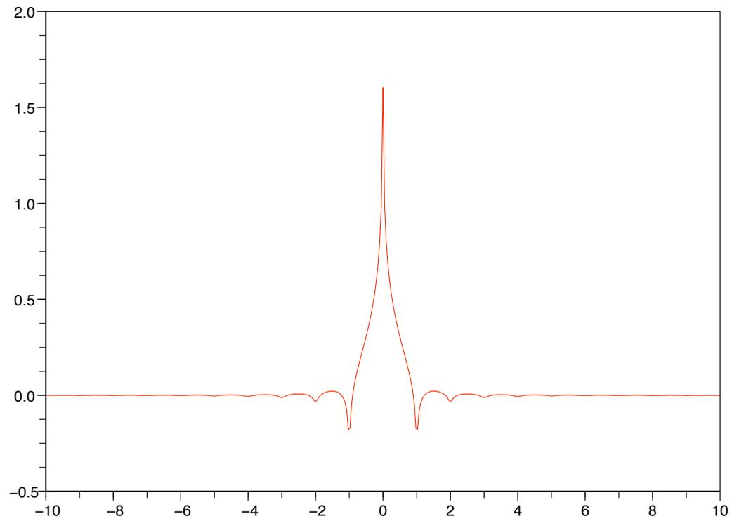
The minimal phase LG counterpart  $\phi$  for  $\mathbb{P}_1$  interpolation
