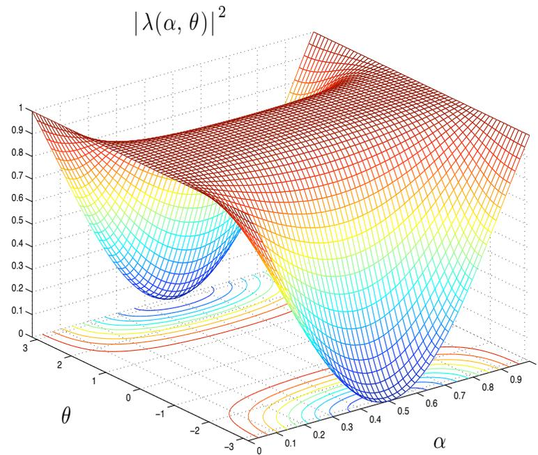
Amplitude of the **amplification factors**  $\lambda$  for cubic interpolation
