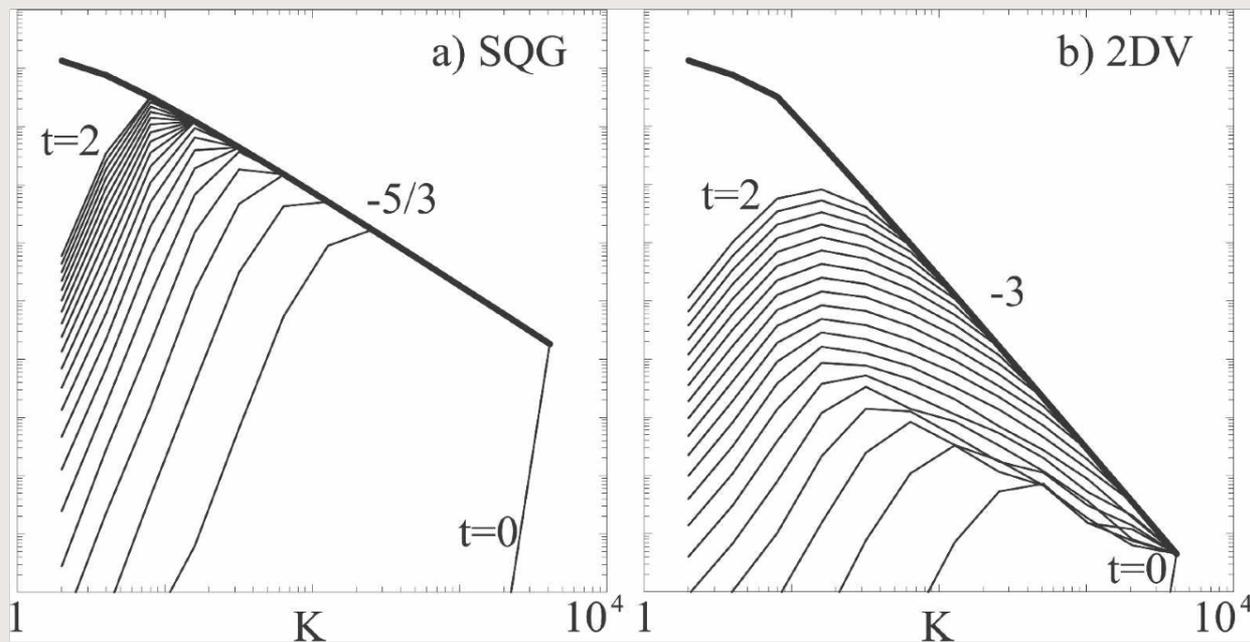
FIG. 1. Error energy per unit wavenumber,  $K^{-1}Z(K, t)$  for  $t = 0, 2$  in steps of 0.1 for (a) SQG turbulence and (b) 2DV turbulence. The heavy solid line indicates the base-state kinetic energy spectra per unit wavenumber,  $K^{-1}X(K)$ , which has a  $-5/3$  slope for SQG and a  $-3$  slope for 2DV.
