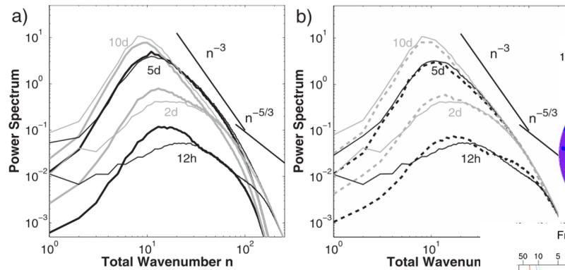
FIG. 8. Power spectrum of the error of the ensemble-mean forecast (thin solid lines) and spread hPa for fixed forecast lead times of 12 h, 2 days, 5 days, and 10 days for (a) the operational ensemble (spread in OPER: thick solid line) and (b) the ensemble system with a stochastic backscatter scheme (spread in SSBS: thick dashed line). SSBS is short for SSBS-FULLDISS. Lead times of 12 h and 5 days are shown in black and for 2 days and 10 days in gray. See text for details.
