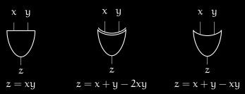
• For the whole circuit, we have one variable for each circuit input bit and each gate output, and one polynomial per gate.
